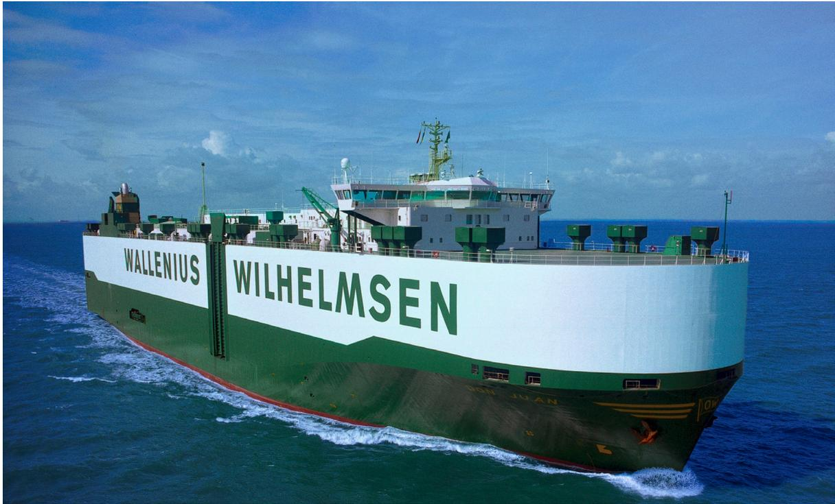
The PCTC (Pure Car Truck Carrier) m/v DON JUAN has a capacity of 5,846 cars or a combination of 2,959 cars and 485 trucks. DON JUAN is a sister ship to TURAN-DOT and TITUS. The ship is built to the highest class of
